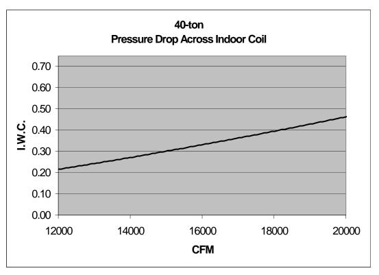
FIGURE 28 - 40 TON - PRESSURE DROP VS. CFM ACROSS INDOOR COIL (DOMESTIC)
